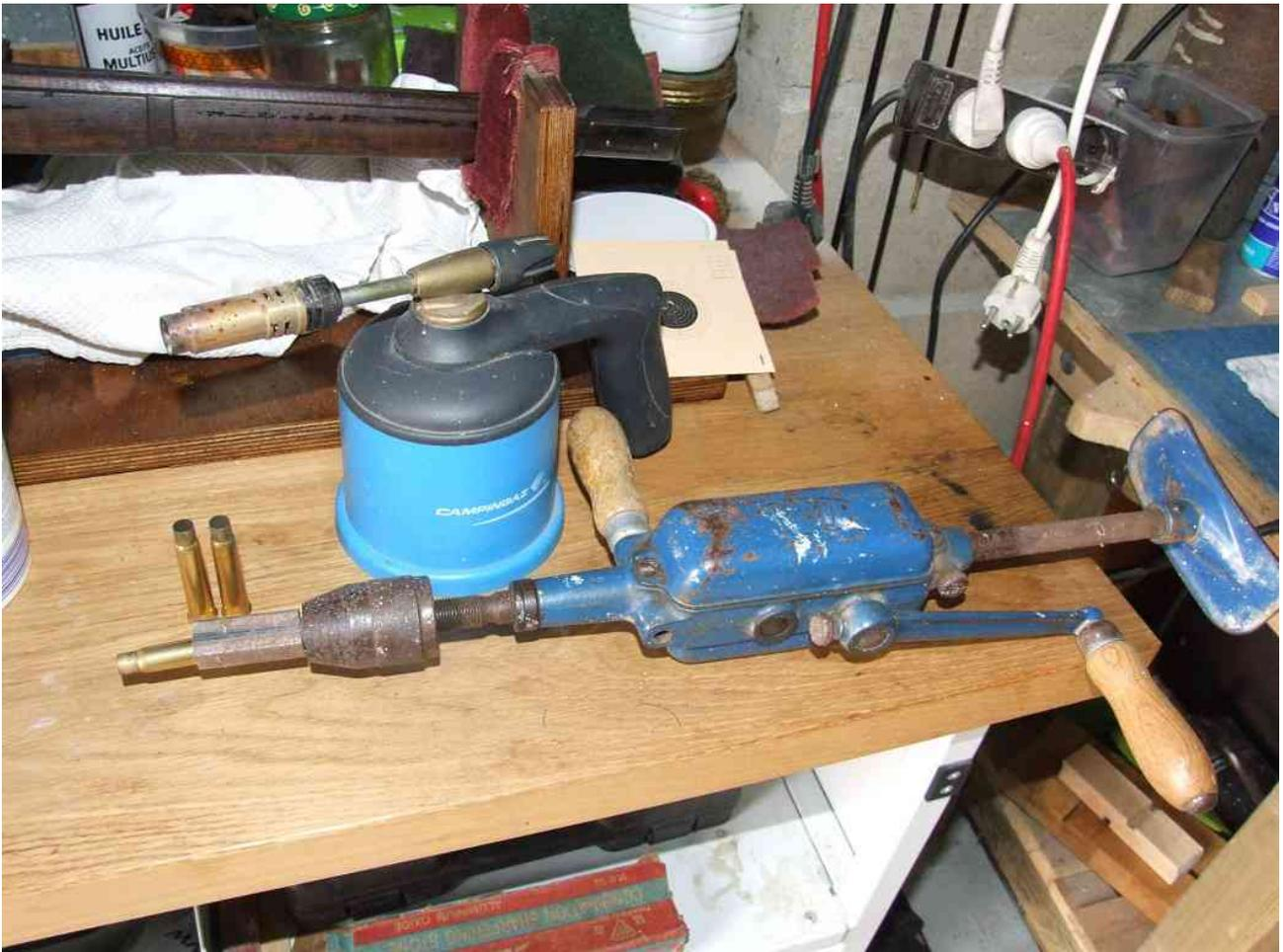
The flame of the blow lamp has an inner and outer cone. The tip of small inner cone is the hottest part of the flame; and also the easiest part to see. Put the neck of the case at the tip of the inner cone and spin the case with the hand drill. The neck will change colour as it heats up; the colour change moves down the case as it heats up. When the colour ring gets to about a neck length below the shoulder; I drop it straight into a bucket of water\*. Then take the next case and repeat.
