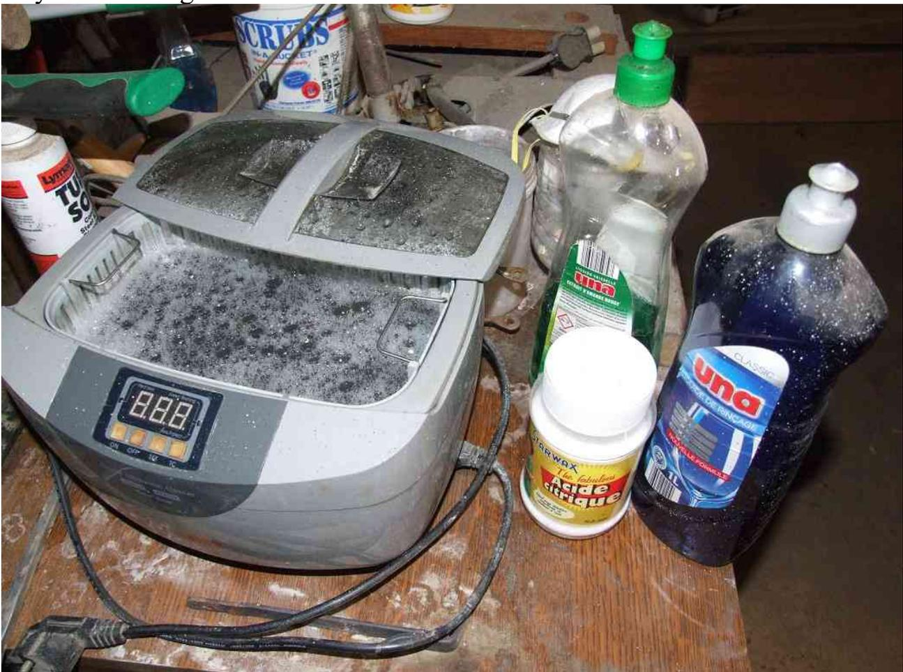
When the cases come out clean; I drop them into warm water with some rinse fluid (to prevent water stains on the brass) in a salad centrifuge basket; move the basket around by hand to flush the cleaning mix off of the cases. The remove the water and spin in the centrifuge to remove excess water before tipping into an old tea cloth to dry off any remaining water droplets.
