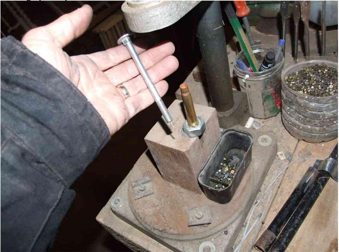
Note: if you bend the pin; you can straighten it once or twice; but better to remove it and fit a new pin. If it breaks, you'll have to drill another coach bolt!
