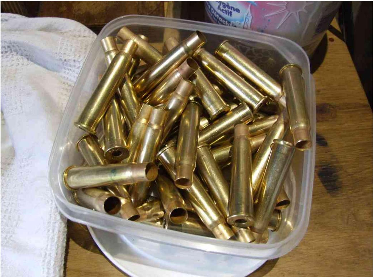
The cases need to completely dry inside before loading; so leave them to dry fully in a warm environment before you attempt to load.
